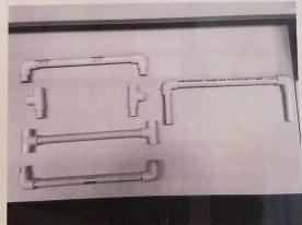
Connect the Elbows to three of the cut 12" PVC pipe bars at both ends.
